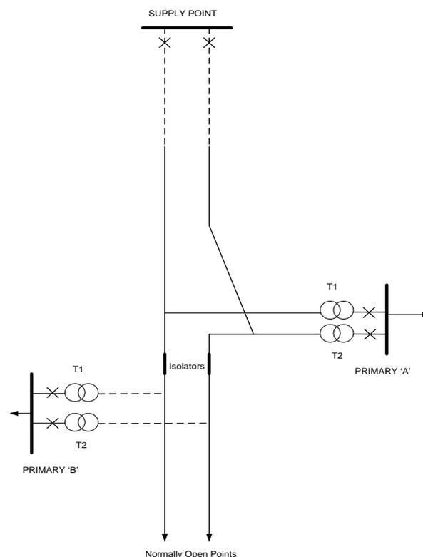
Figure 1 – Schematic of supply circuits
