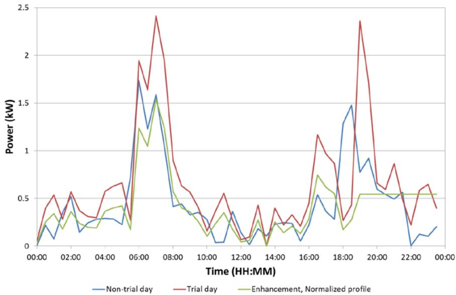
**Figure 10 Mean Trial Day, Non-trial day and Enhancement, Normalized profile ASHP profiles**
