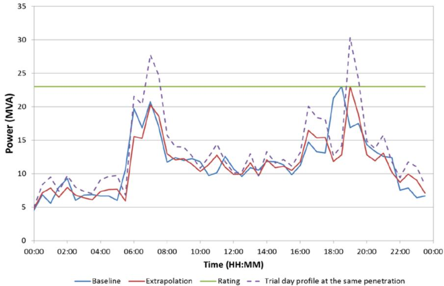
**Figure 9 Baseline (*Non-trial Day*), Extrapolation (*Trial Day*) and *Trial Day* profile at the same penetration as the Baseline (Rise Carr load + trial day profile \* baseline ASHP number 8478)**
