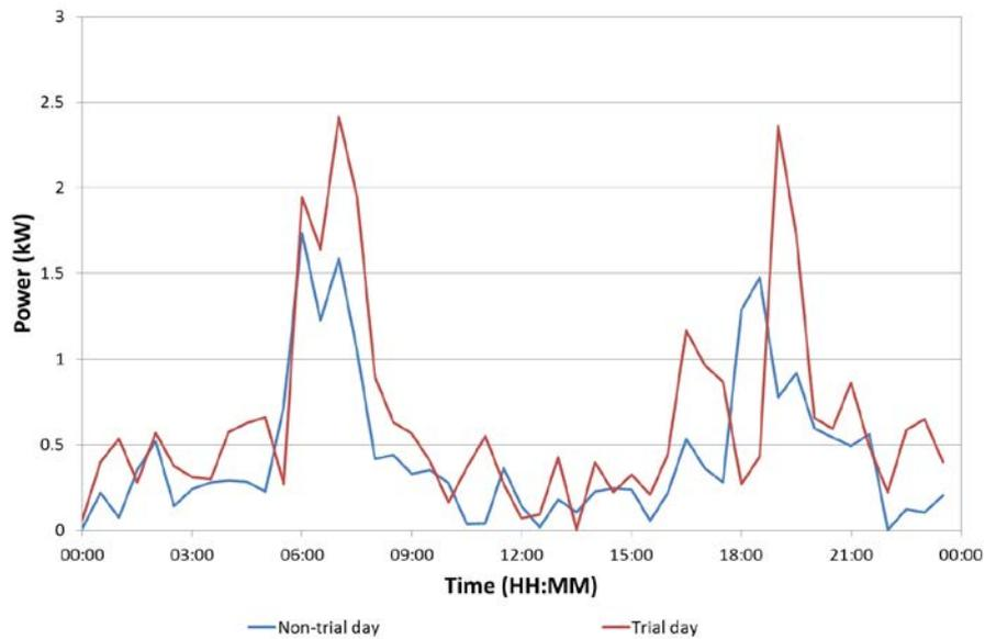
Figure 4 Mean *Trial Day* and *Non-trial day* ASHP profiles
