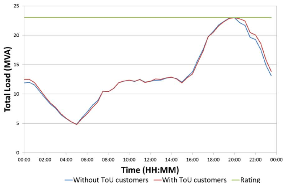
Figure 7 Load Profiles of Rise Carr Network EV with and without TOU customers downstream
