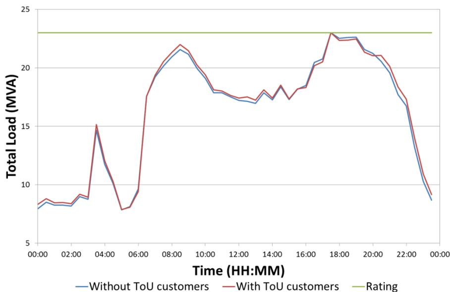
Figure 8 Load Profiles of Rise Carr Network ASHP when DSR is applied or not
