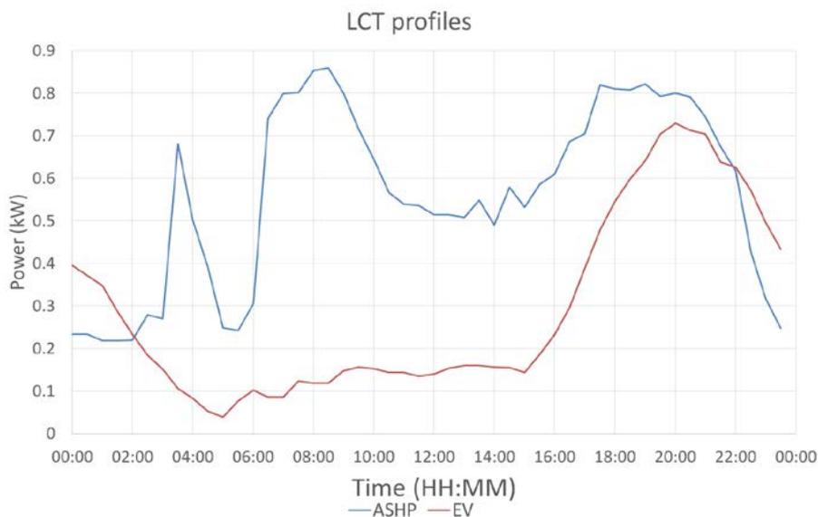
Figure 6 ASHP and EV mean daily consumption profiles from CLNR trial data [8, 9]
