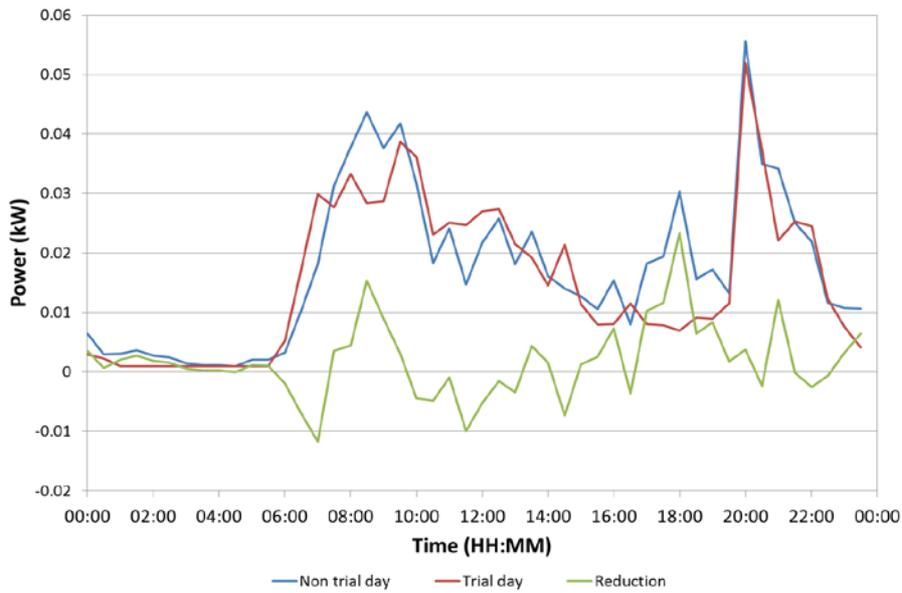
Figure 5 Domestic washing machine load profile
