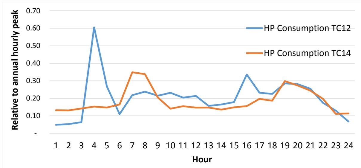
**Figure 7: Heat pump consumption comparison between TC12 and TC14; annual average profiles**
